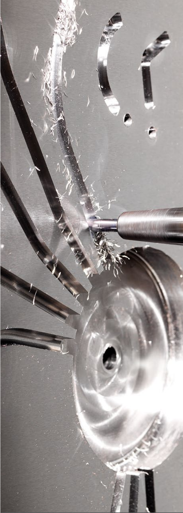
CS Tool's investment in an a82 horizontal machining center helped the company employ production machining practices in its own mold-making processes to improve workflow flexibility and throughput.
