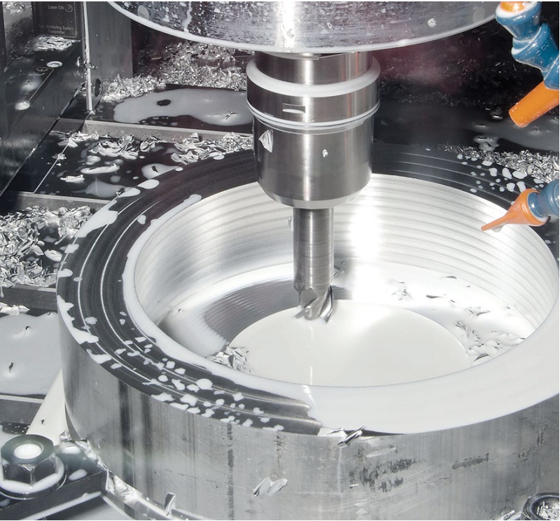
The V56i has enabled Fallbrook to easily hold profile tolerances and achieve finishes of 0.2 micron Ra or less.
